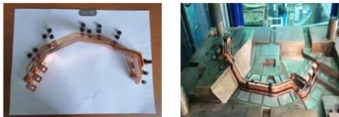
(a) Clip assembly (b) Busbar loading
