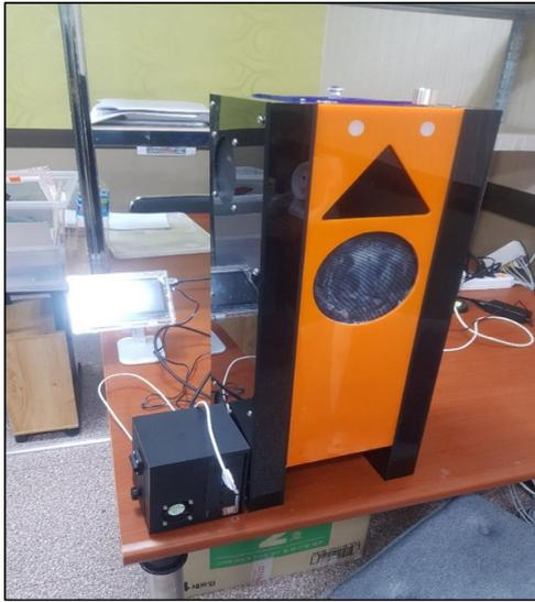
Fig. 2. Photograph of air sterilizer operated by electrolytic salt catalyst.
