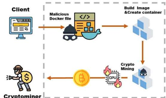
(Figure 5) Malicious Docker File-Based Crypto Jacking Mechanism
