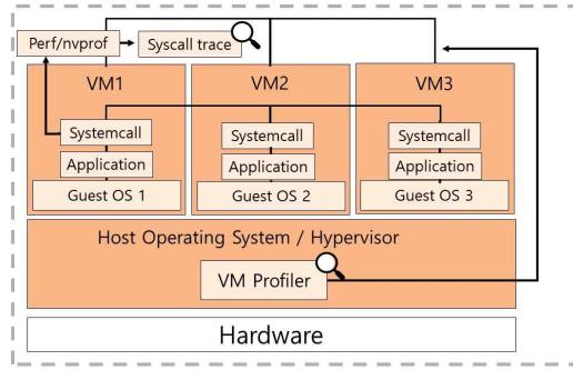
(Figure 2) Diagram of Virtual Machine-Based Environment
