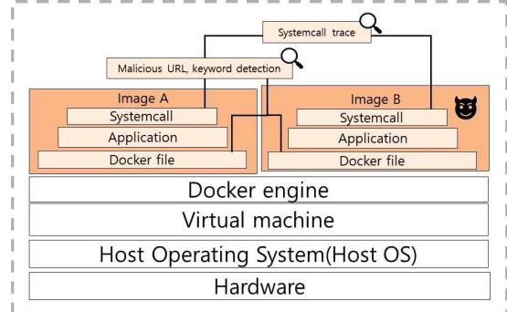
(Figure 1) Diagram of Container-Based Environment
