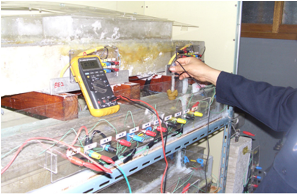
Fig. 2. View of potential measurement of reinforced concrete specimen
