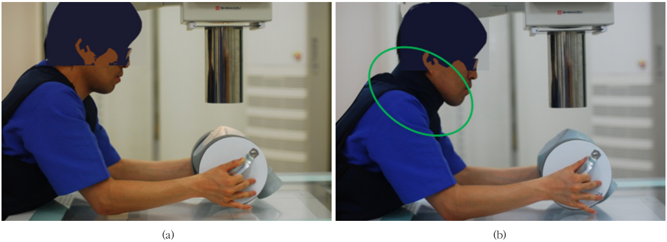
Fig. 3. (a) Measurement of thyroid radiation dose in human model (without thyroid radiation shielding) (b) Measurement of thyroid radiation dose in human model (including thyroid radiation shielding)
