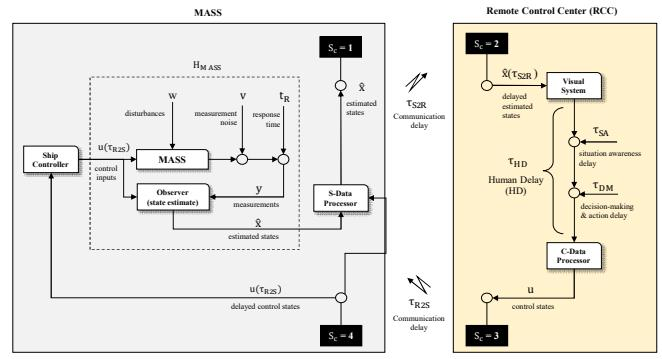
Fig. 1 Remote control model
