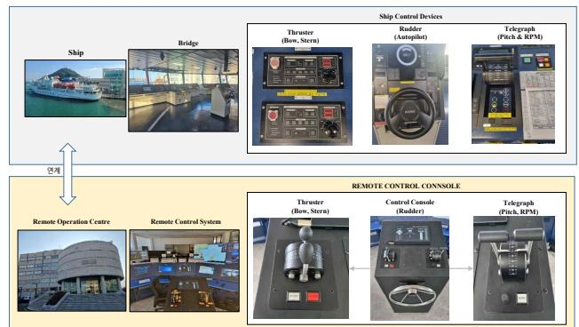
Fig. 2 Ship's control devices(upper) and remote control devices(lower)
