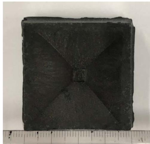
Fig. 3. YBa<sub>2</sub>Cu<sub>3</sub>O<sub>7</sub> superconducting bulk by top seeded melt growth.
