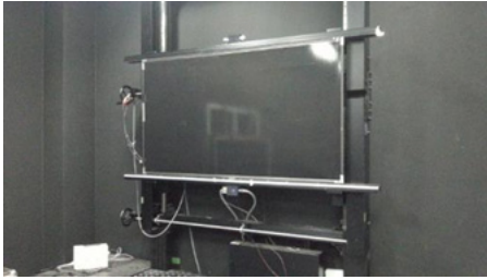
Fig. 4. Long-pulse type solar simulator with CIGS test module
