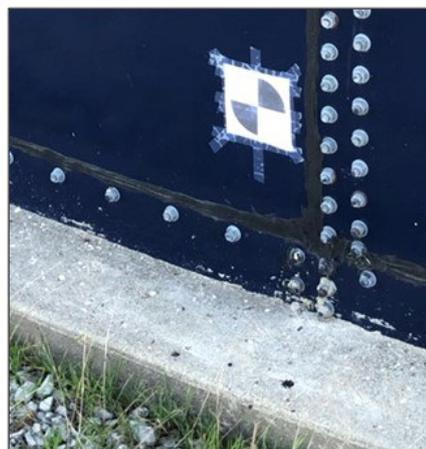
Fig. 4. A georeferencing checkerboard paper target on Tank-2 structure.
