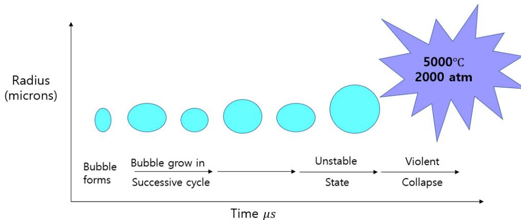
Fig. 1. Time-dependent ultrasound-based cavitation (Pilli et al., 2011)
