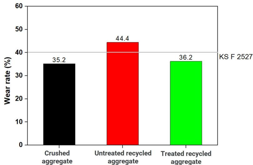
Fig. 8. Wear rate test results
