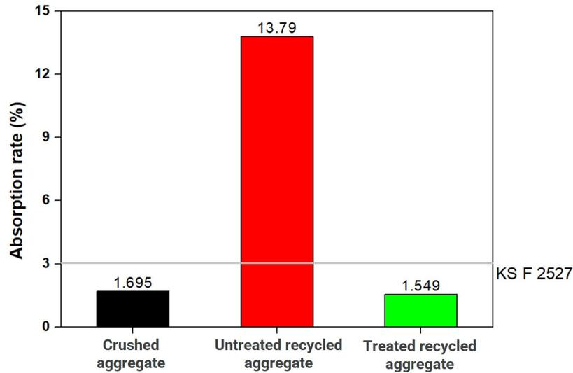
Fig. 7. Absorption rate test results
