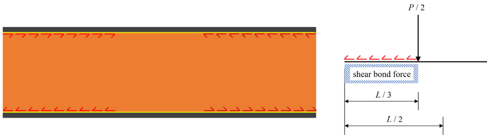
Figure 2. Shear force distribution by shear flow
