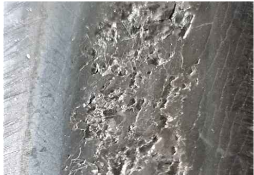
(a) Rail surface defects in acceleration section
