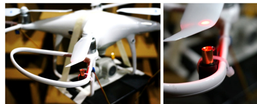
Fig. 1. (Color available online) Experimental setup for analysis of the acoustic characteristic of a quadcopter.
