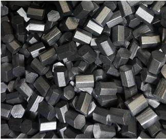
Fig. 6. Shape of propellant
