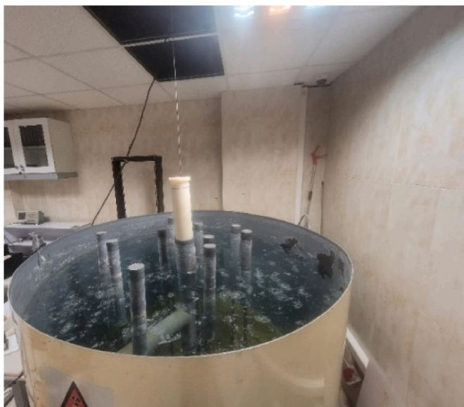
Fig. 2. Am–Be source is placed at the center of the iron tank containing water.
