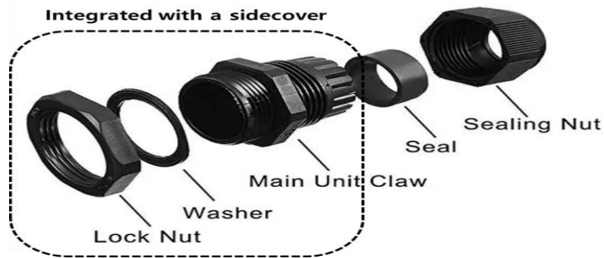
Figure 2. Structure of cable gland parts for the AC power cord
