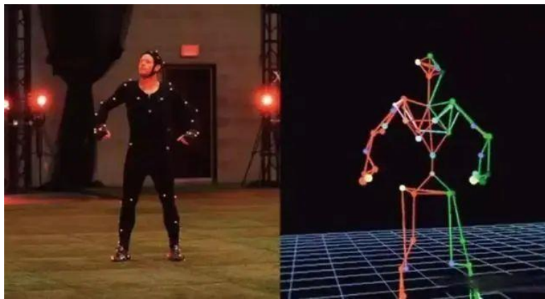
Figure 1. Motion capture in film and Television Production Involves Identifying Joint Positioning Points for Motion Tracking.
