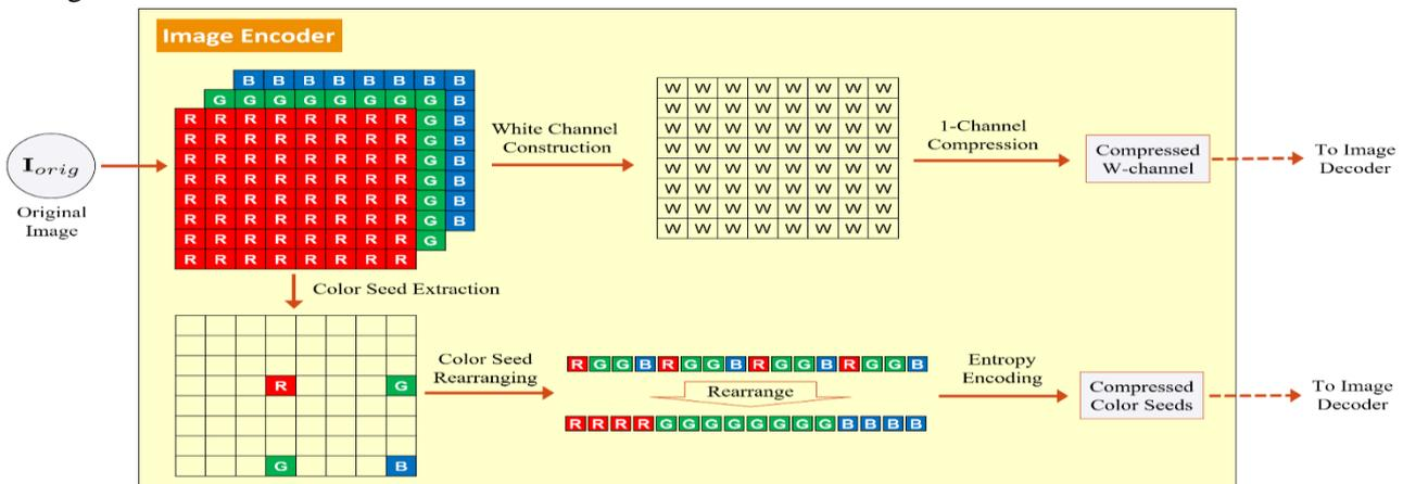
Figure 1. Diagram of the proposed Encoder
