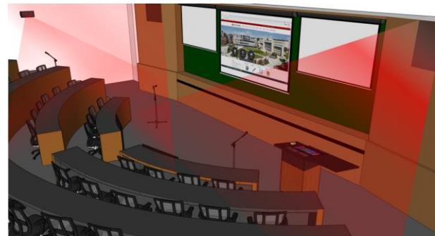
(b) 3D model for measuring pink noise in the field
