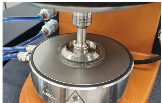
Fig. 3 Compression test. Hyaluronic acid fillers were put at the center of plate of rheometer.
