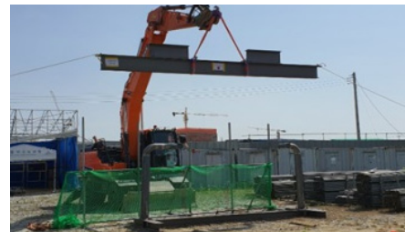
Fig. 4. Impact test on self-supporting drop safety device.
