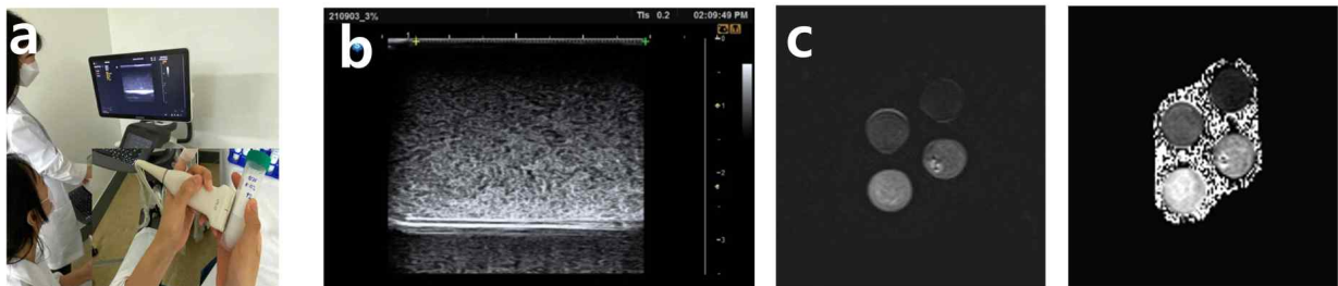
Fig. 1. Ultrasound data acquisition process and magnetic resonance 6-point Dixon imaging of simulated fatty liver phantom. (a) Acquisition of ultrasound images of simulated fatty liver phantom, (b) Ultrasound imaging of a 3% water-oil phantom, (c) 6-point Dixon MRI, the left is fat only image and right is fat percentage image.
