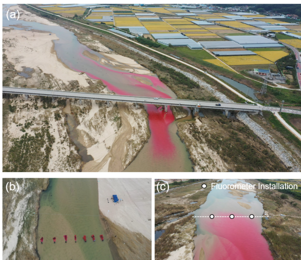
Fig. 4. Tracer cloud shape flowing along a river channel at Gam Creek, South Korea
