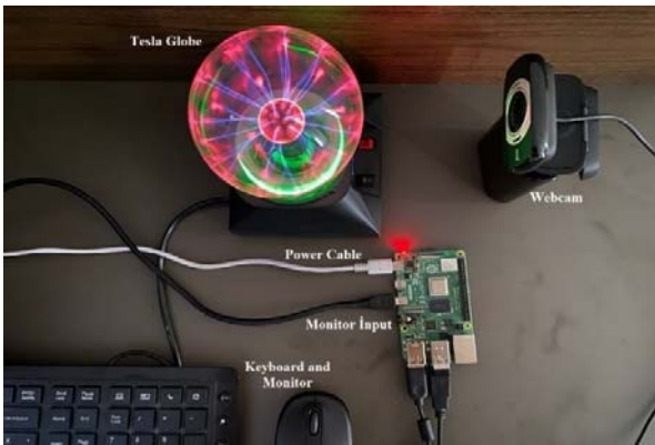
Figure 8. General view of the webcam sensor system.
