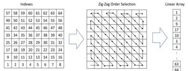
Figure 5: Zig-Zag selection of 2-D Coefficients for Linear Array
