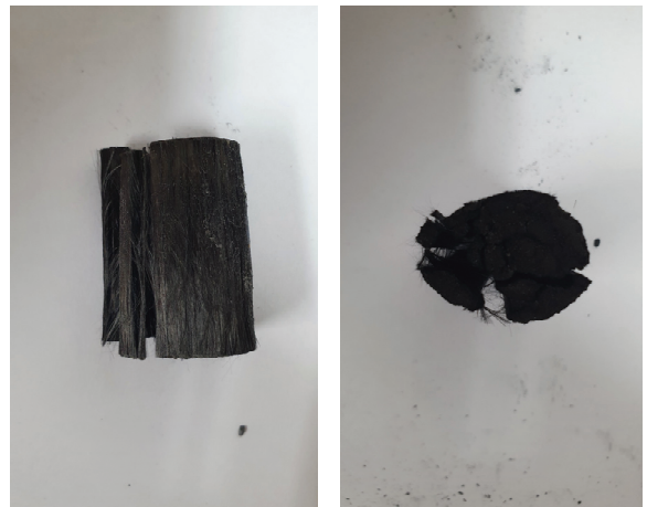
Fig. 8. CFRP resin loss due to high temperature in compressive test object
