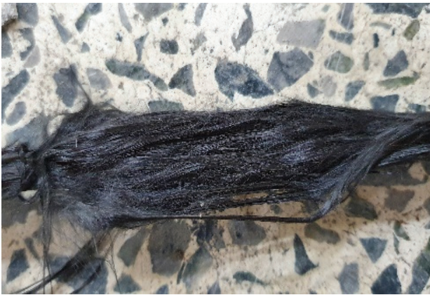
Fig. 6. CFRP resin loss due to high temperature in tensile test object
