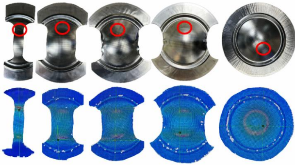
Fig. 13 Specimens and ARGUS measurement results
