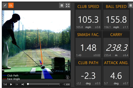
<Fig. 5> Swing and ball trajectory measuring equipment (Trackman)
