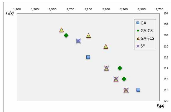
Fig. 5 Pareto Optimal Solutions of Each Approach in Problem 3 of Scale 3
