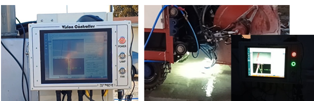
Fig. 4 A control box and A light module of vision system.
