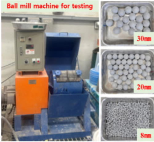
Fig. 2. Ball Mill as a Crushing Device
