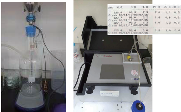
Fig. 2 Particle measurement devices (left) gravimetric method (right) particle counter
