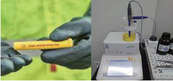
Fig. 3 water measure devices (left) Shell water detector[11] (right) Karl Fischer coulometer
