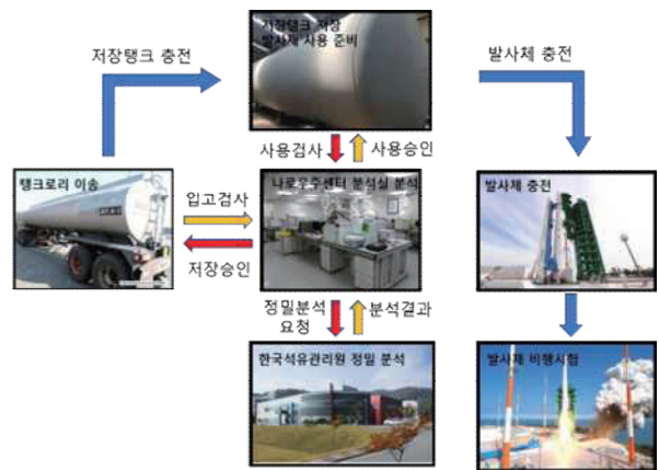
Fig. 8 Procedure of request, inspection and approval of fuel use
