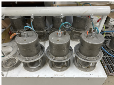
(a) Permeability test
