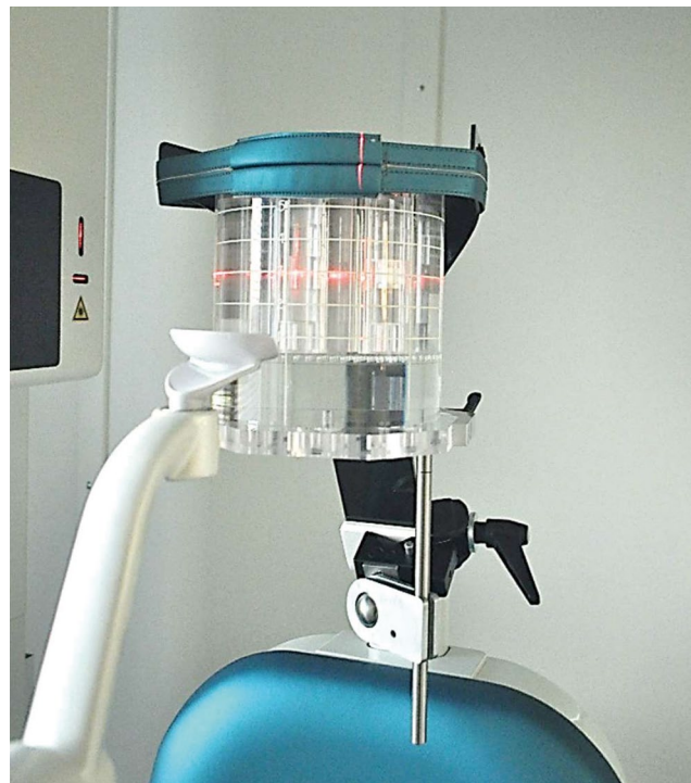
Fig. 1. SedentexCT IQ phantom fixed with a custom-made apparatus.
