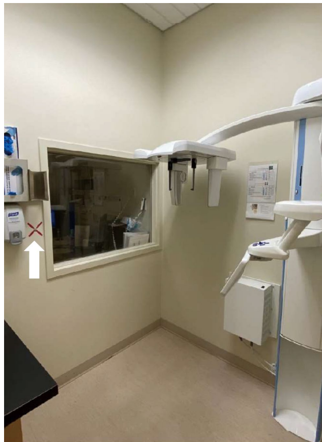
Fig. 1. Photograph of the dental panoramic radiographic unit facing the adjacent room through the lead-glass window, from which the exposure is acquired. The photograph was taken from the doorway, which features a sliding door that is fully closed during the exposure. The patient is instructed to focus on the red cross immediately adjacent to the window for the duration of the procedure.
