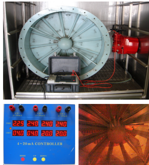
[Fig. 7] Environmental test apparatus for vane damper
