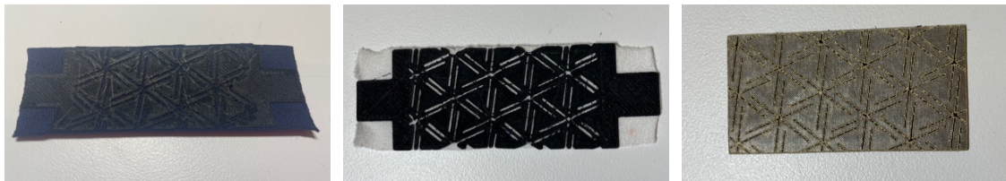
Fig. 4. 3D Printed and laser cut sensor samples (P1B 3D Print, P1W 3D Print, P1B Laser cut).
