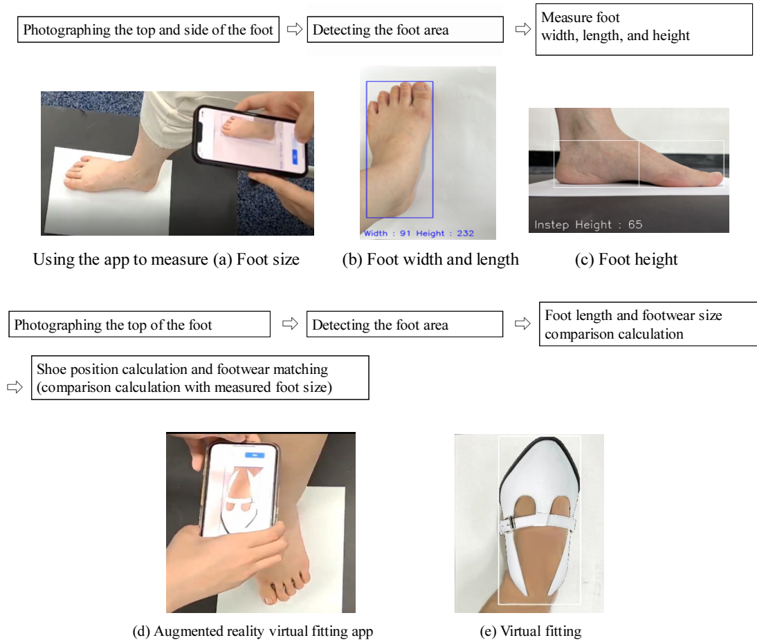
Fig. 2. Foot measurement and use of the AR virtual fitting app.
