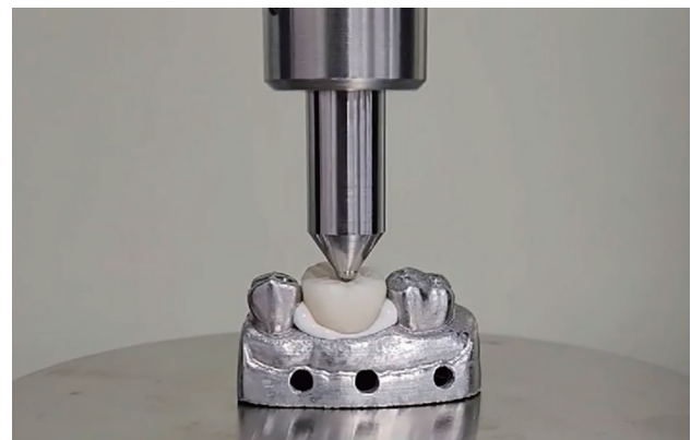
Fig. 4. Fracture strength evaluation using a universal testing machine.
