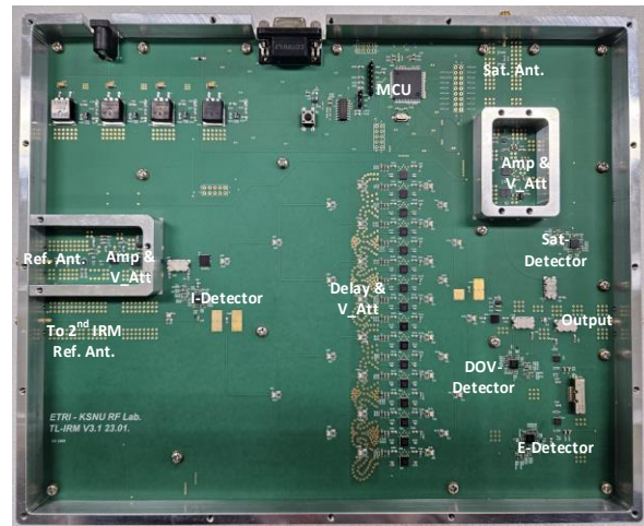
Figure 2. Photo of the Implemented RF IRM
