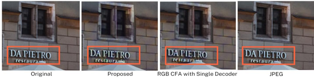
Figure 9. Enlarged Qualitative Comparison of the proposed method with the method using the conventional Bayer CFA with a single decoder for the 3:1 compression rate. Together with the lossless Hoffman encoding, the compression rate becomes 6:1.
