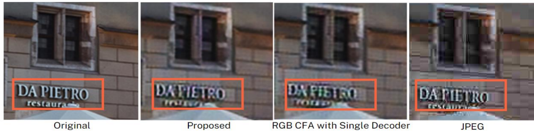
Figure 10. Enlarged Qualitative Comparison of the proposed method with the method using the conventional Bayer CFA with a single decoder for the 12:1 compression rate. Together with the lossless Hoffman encoding, the compression rate becomes 24:1.
