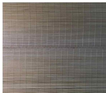
Fig. 9. Staggered arrangement of the chain line of Korean screen for papermaking.
