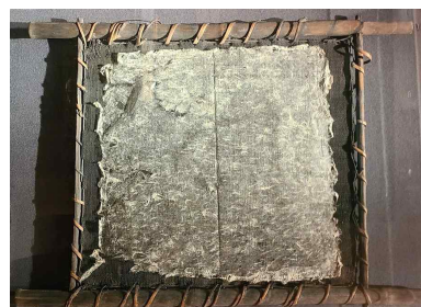
Fig. 3. A primitive papermaking mold with woven cloth. Photo taken by the author in May 2022 at the Robert C. Williams Museum of Papermaking, Atlanta, USA.
