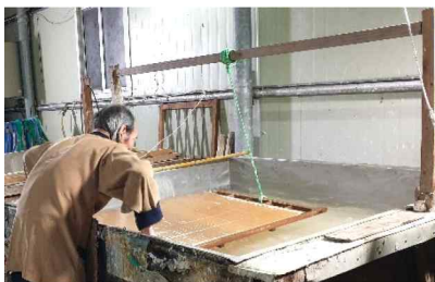
Fig. 11. A Heulimtteugi scene using a mold hanging on the cross bar.
