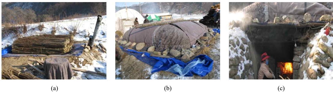
Fig. 2. A modern Daknamu steaming facility using an ondol-type floor. (a) Pile of Daknamu shoots, (b) covered Daknamu pile, (c) fireplace.
