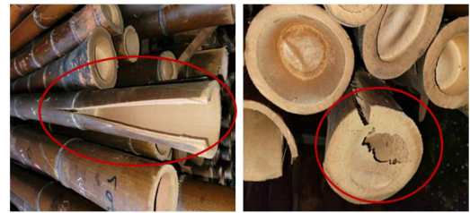
Fig. 8. End checks occurred at both ends of the bamboo poles.
