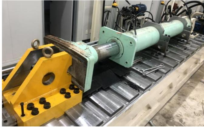
Fig. 7. Compression testing system of a thrust jack specimen
