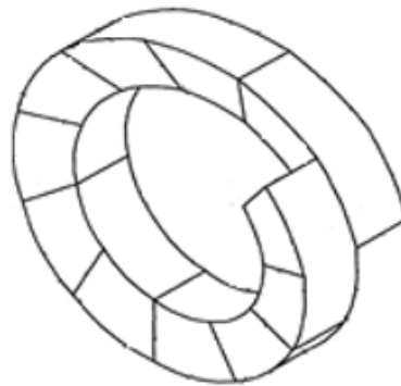
Fig. 8. Design method of helical segment (DE 102009013527 A1, EP 2230380 A2, Herrenknecht, 2010)
