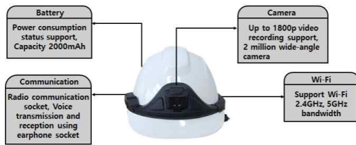
Fig. 2. Composition of smart helmet
