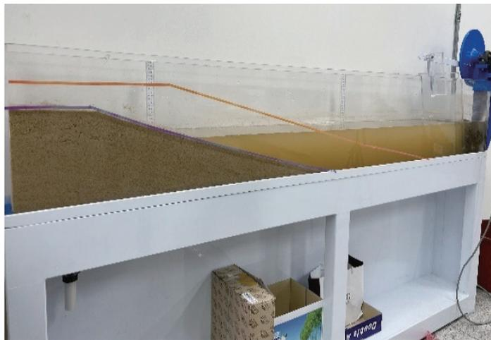
Figure 1. Picture of wave flume before the experiment.
