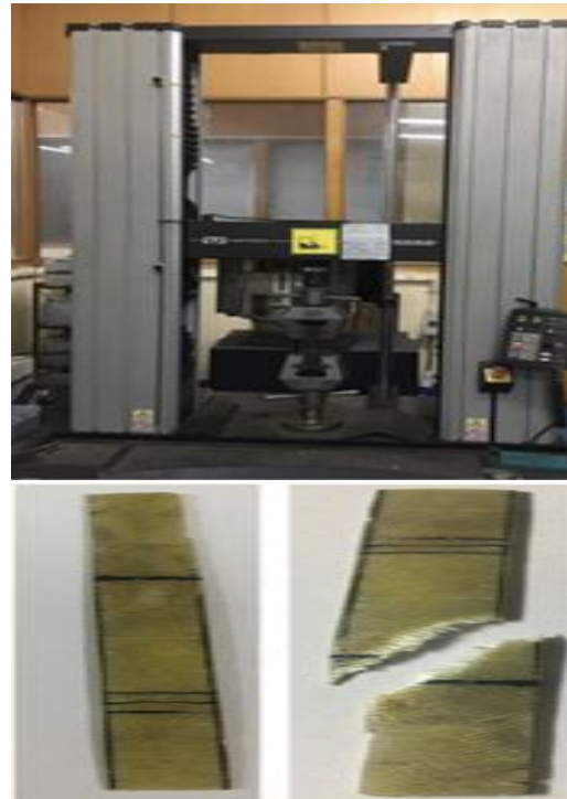
Fig. 4. (a) Universal Tensile Machine(top) Bottom Fig 4(b) Types of delamination and Fractured surface of the untreated composite before and after tensile loading of GFRP-EP3 composite.
