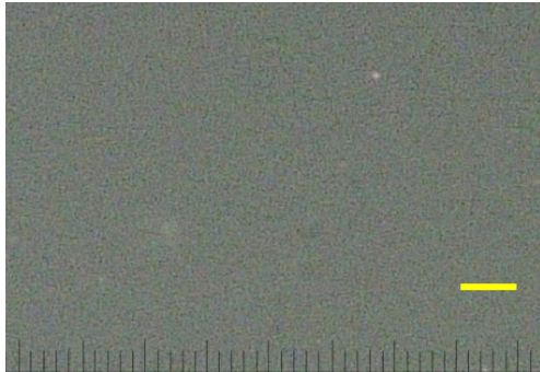
Fig.10. Hematite particles flowed out during magnetic separation with a triangular cross-section filter. Almost no particles were found. (Scale is 10 \mu m.)
