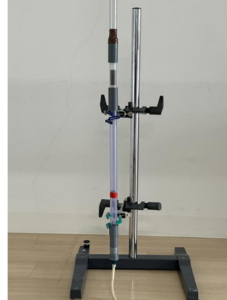
Fig. 3. Piping for magnetic separation. Developed magnetic separation filter is placed in the center.
