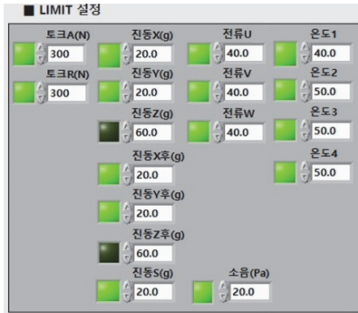
Fig. 9 Vibration and temperature sensor criteria setting
